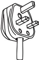
This appliance must be grounded. In the event of an electrical short circuit, grounding reduces the risk of electric shock by providing an escape wire for the electric current. This appliance is equipped with a cord having a grounding wire with a grounding plug. The plug must be plugged into an outlet that is properly installed and grounded.
